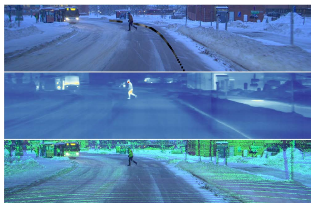
Figure 4. An example frame from the collected dataset. On top, there is an RGB camera image with the overlaid road weather sensor data, where darker colour means a higher grip, at the centre there is a fused thermal camera image, and at the bottom, the LiDAR reflectance data is overlaid on the RGB camera image.
