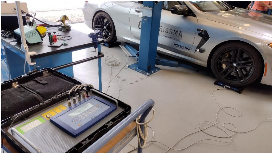
Figure 21. Measurement of the longitudinal and lateral position of the CG.
