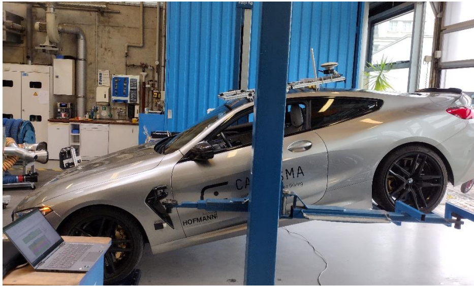
Figure 22. Measurement of vertical position of the CG.
