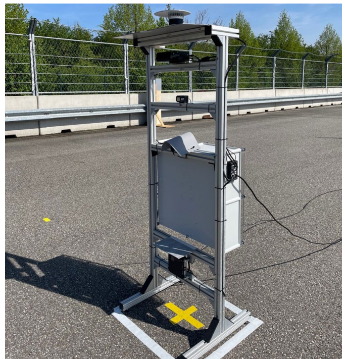
Figure 1. Data capture setup with REHEARSE sensors at the CARISSMA's Outdoor Track, featuring a layered arrangement of devices: a Rotative LiDAR (top), followed by MEMS, LiDAR, RGB and FLIR cameras, and a 4D RADAR.
