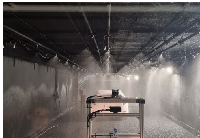
Figure 3. Cerema's PAVIN platform simulating rain
