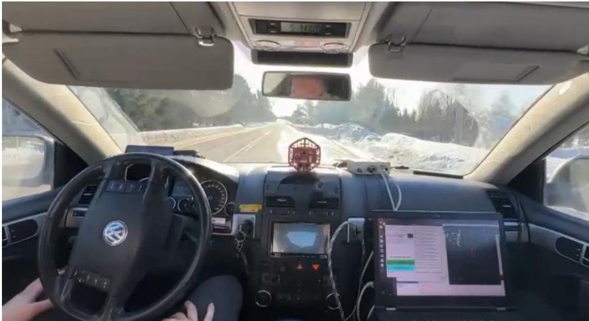
Figure 10: MRM execution from automated driving mode (recorded inside the VTT vehicle).
