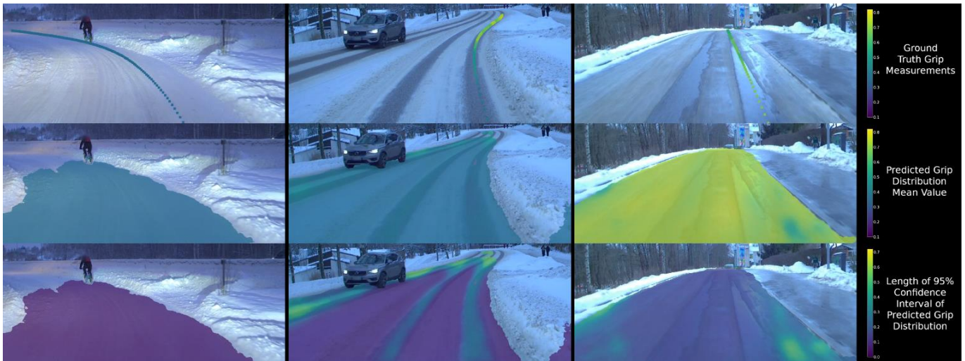
Figure 6: Three example frames on grip prediction and road area segmentation.
