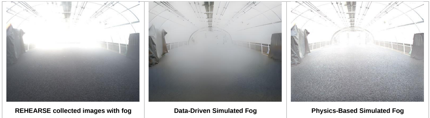
Figure 23: Comparison of 30m visibility fog in the collected data and ROADVIEW fog models
