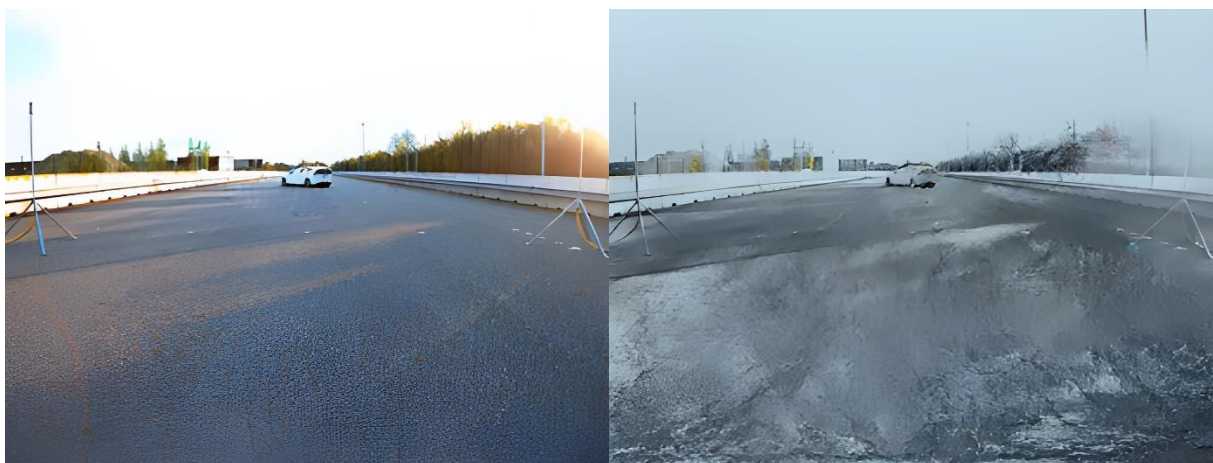
Figure 24: Images generated by the data-driven snow model for validation. Left: light snow, Right: heavy snow
