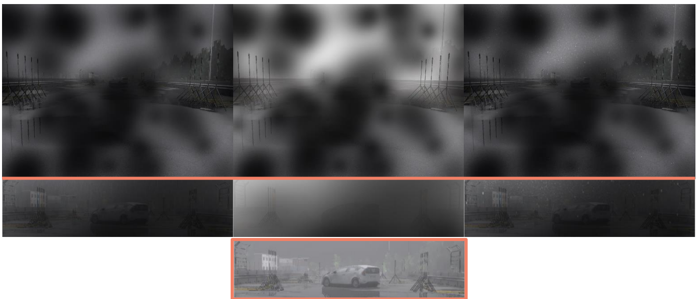
Figure 16: Weather model compounded with a lens soiling model. Left: Rain. Middle: Fog. Right: Snow. Middle row: zoomed in area of the frame. Bottom row, corresponding zoomed area in the original image.
