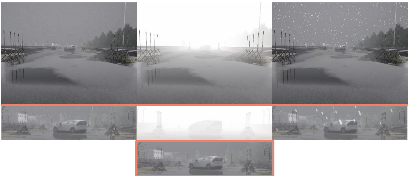
Figure 21: Weather model compounded with a wind model. Left: Rain. Middle: Fog. Right: Snow. Middle row: zoomed in area of the frame. Bottom row, corresponding zoomed area in the original image.
