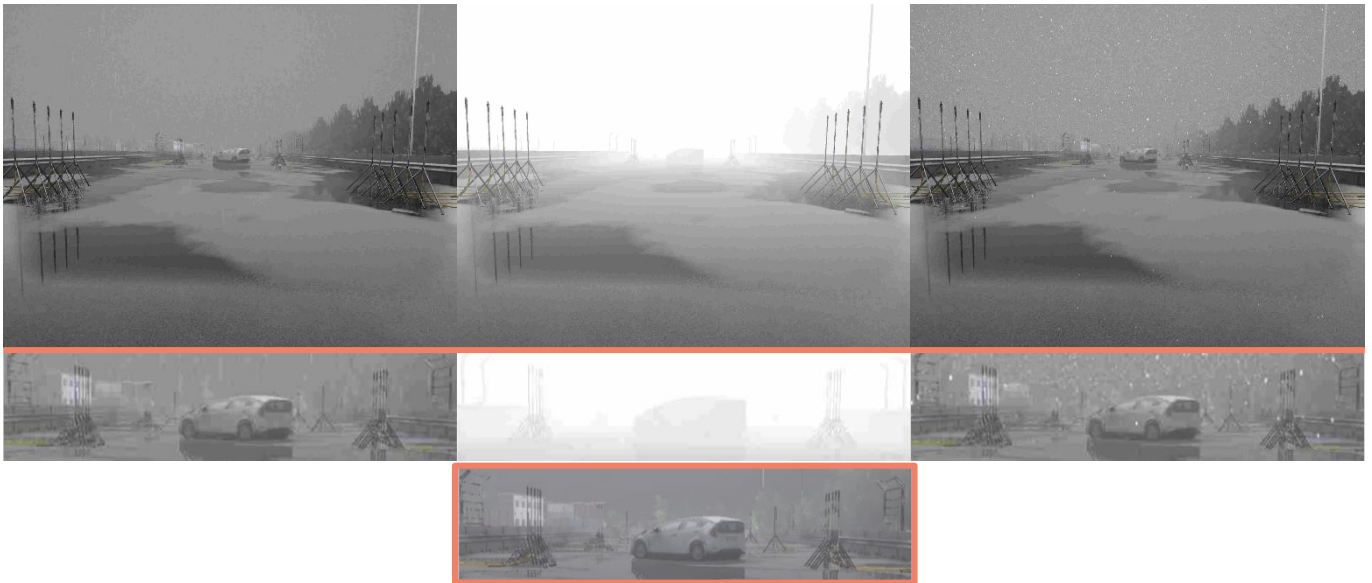
Figure 19: Weather model compounded with lossy compression. Left: Rain. Middle: Fog. Right: Snow, Middle row: zoomed in area of the frame. Bottom row, corresponding zoomed area in the original image.
