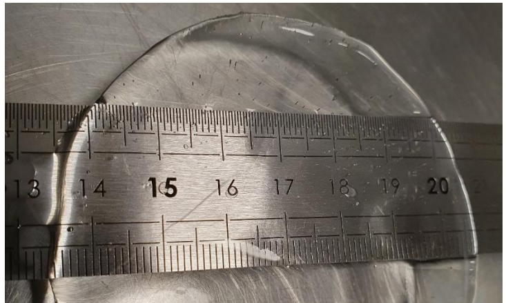
Figure 5. A disc of clear ice on a steel ruler. The surface is wet. A few air bubble impurities are seen.
