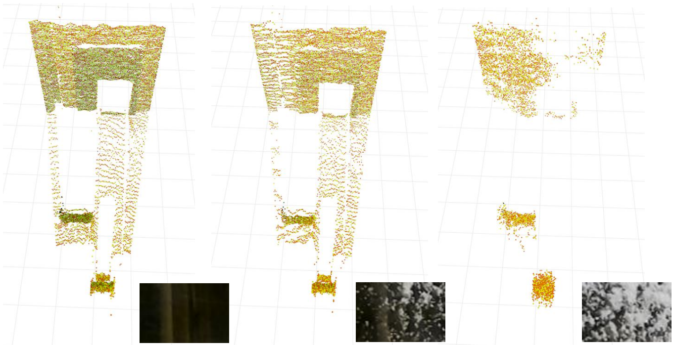
Figure 6. Example of point clouds from single scans, from no snow (left) over 2/5 to about 4/5 covered (right).
