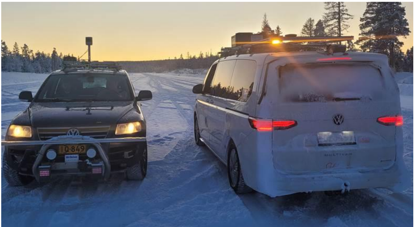
Figure 27. Test vehicles from VTT in dry snow in cold winter conditions. Snow did not stick to the top mounted lidar of the left vehicle. Aerodynamic effects makes spray snow stick on the back of the right vehicle.
