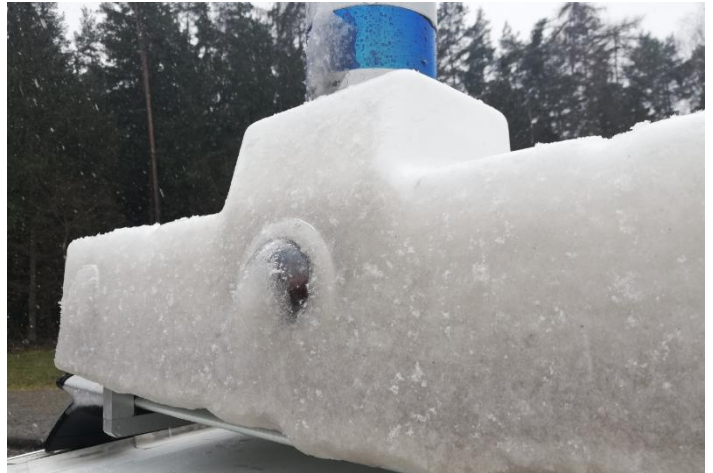
Figure 26. Snow on AVL's sensor rack on the roof of their test vehicle. The VLP-32 lidar is covered in snow on the side facing the vehicle's direction of travel. The camera dome below is also covered.
