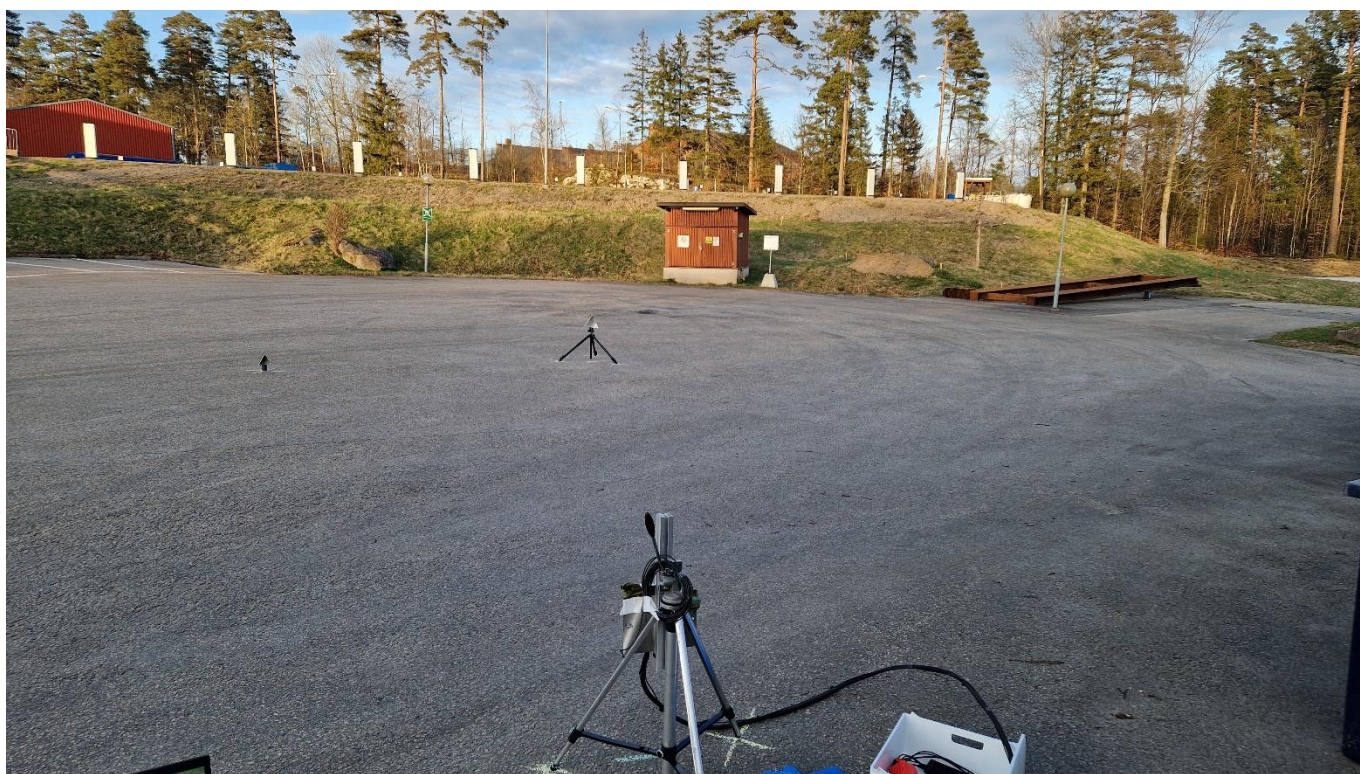
Figure 21. Radar mounted on stand at parking lot. The two reference corner reflector targets can be seen further away on the flat asphalt space.
