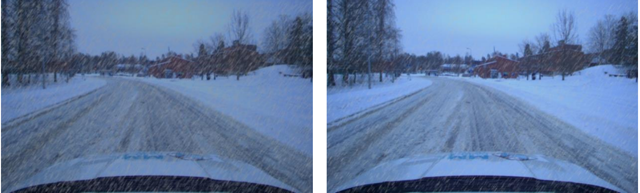
Figure 3. Rain distortion, Left droplet share = 0.007 & brightness 0.7. Right: droplet share = 0.003, brightness 0.9
