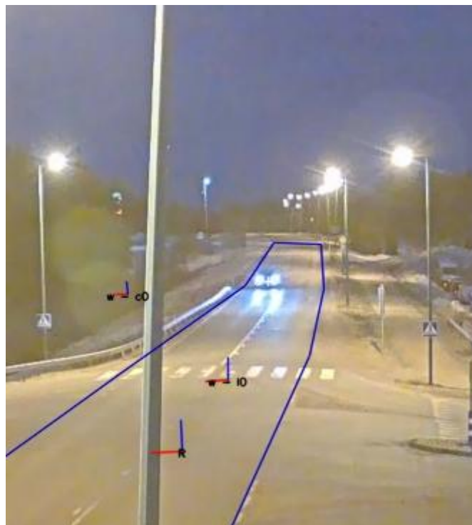
Figure 35: Vehicle not detected in the top part of the road – nightlight.
