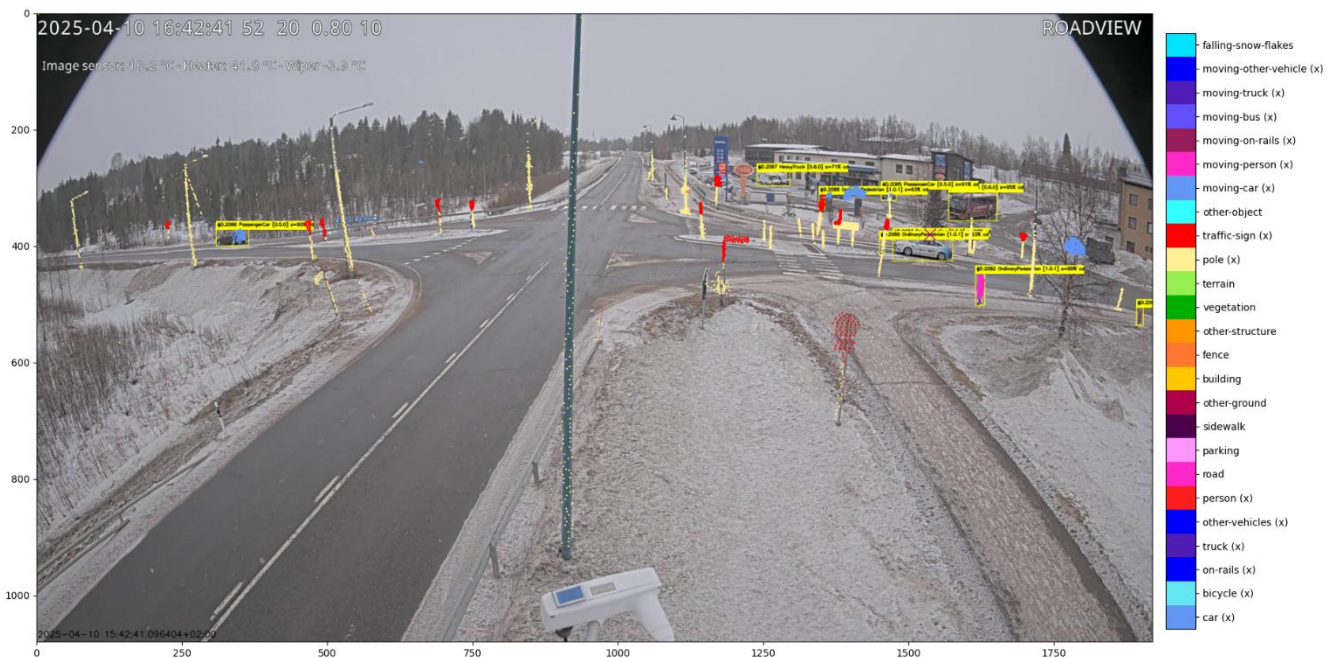
Figure 41: Combined perception of FGI's LiDAR and CRF's camera, with a pedestrian detected by both sensors.
