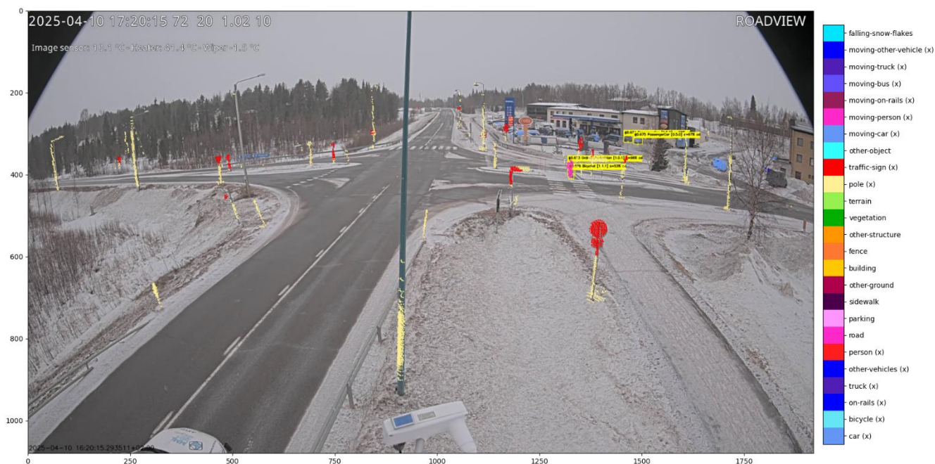
Figure 46: Different perception results between roadside's camera and vehicle's LiDAR.
