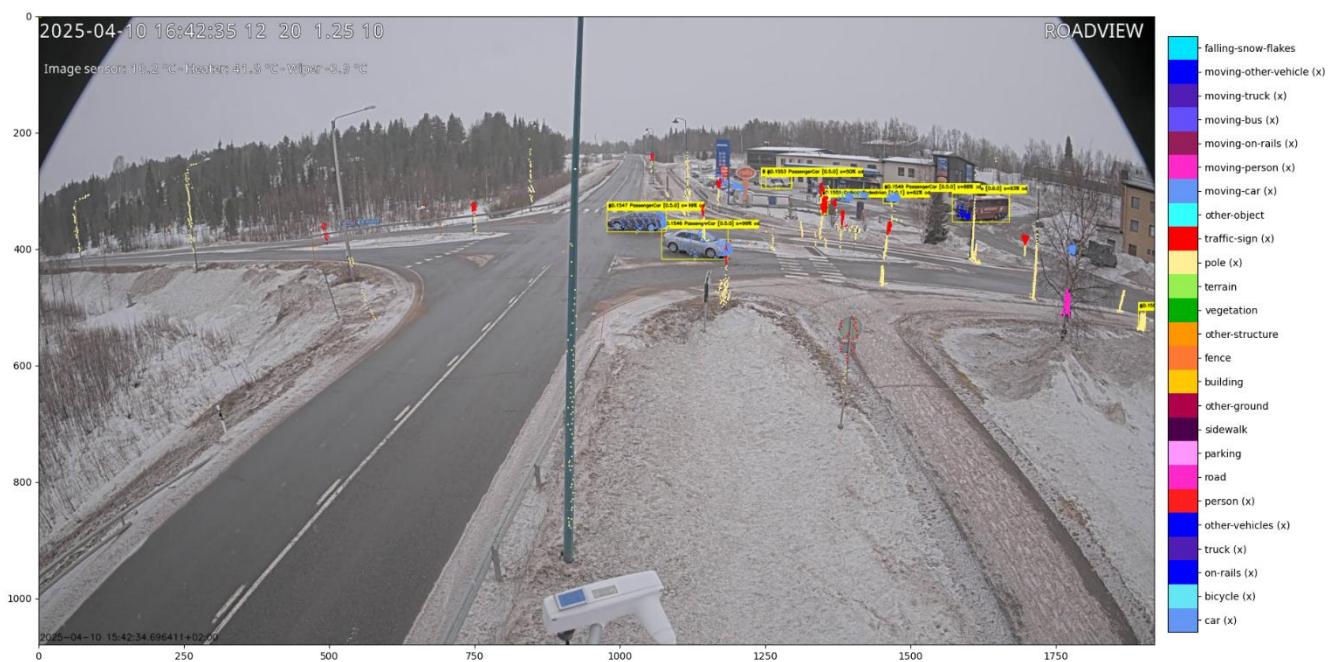
Figure 43: Combined perception of FGI's LiDAR and CRF's camera, with a pedestrian only detected by FGI's LiDAR.
