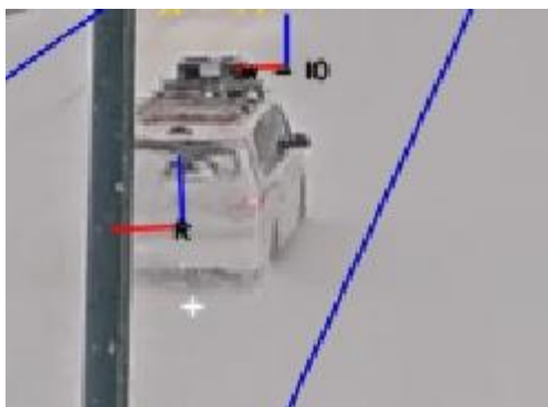
(a) vehicle not detected by the camera-based perception
