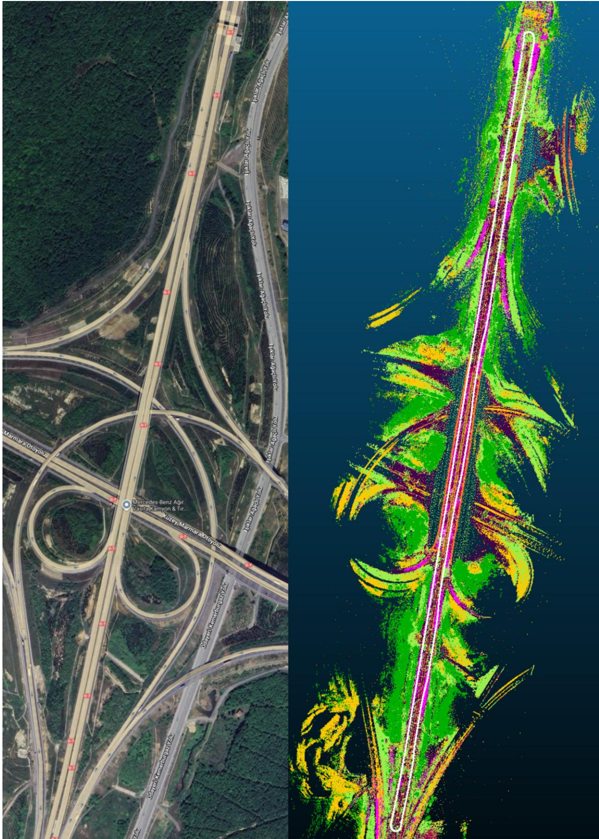
Figure 5. A map of the Turkish Highway is shown on the left side (© Google) and graph-optimized semantically segmented point cloud data of the same area is shown on the right. The driven test trajectory is depicted in white color.
